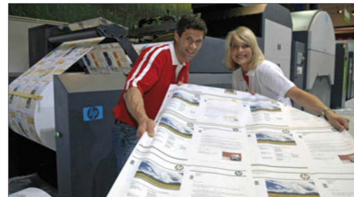
The press is capable of printing up to 2,600 letter-size pages per minutes
